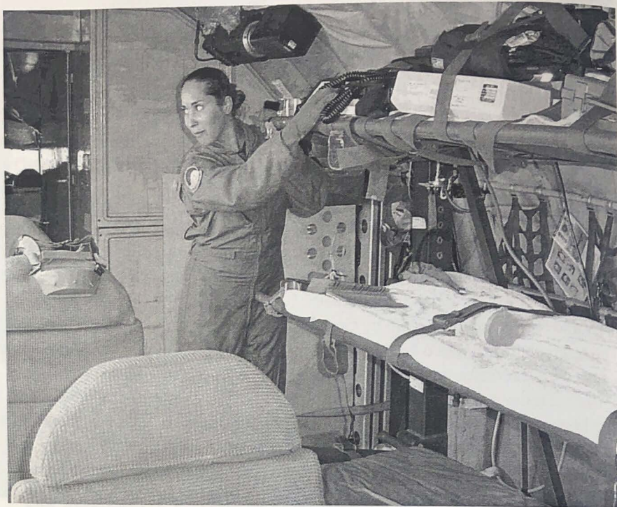
A medical technician from Travis AFB, Calif., sets up a Patient Support Pallet prior to receiving patients. Each PSP contains three litters and three seats, with room for additional medical equipment.
